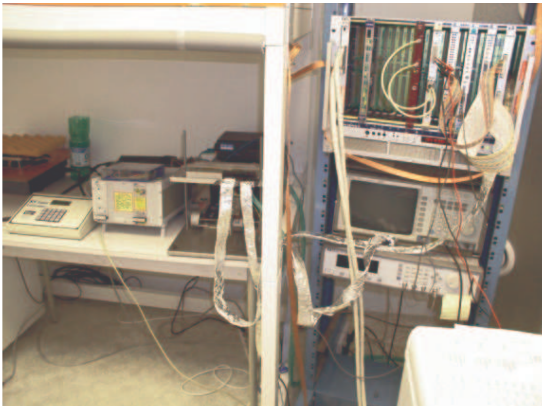
Figure 6. Readout system in VME crate (left) and place for beta source test and laser test setup with XY stage (right)
