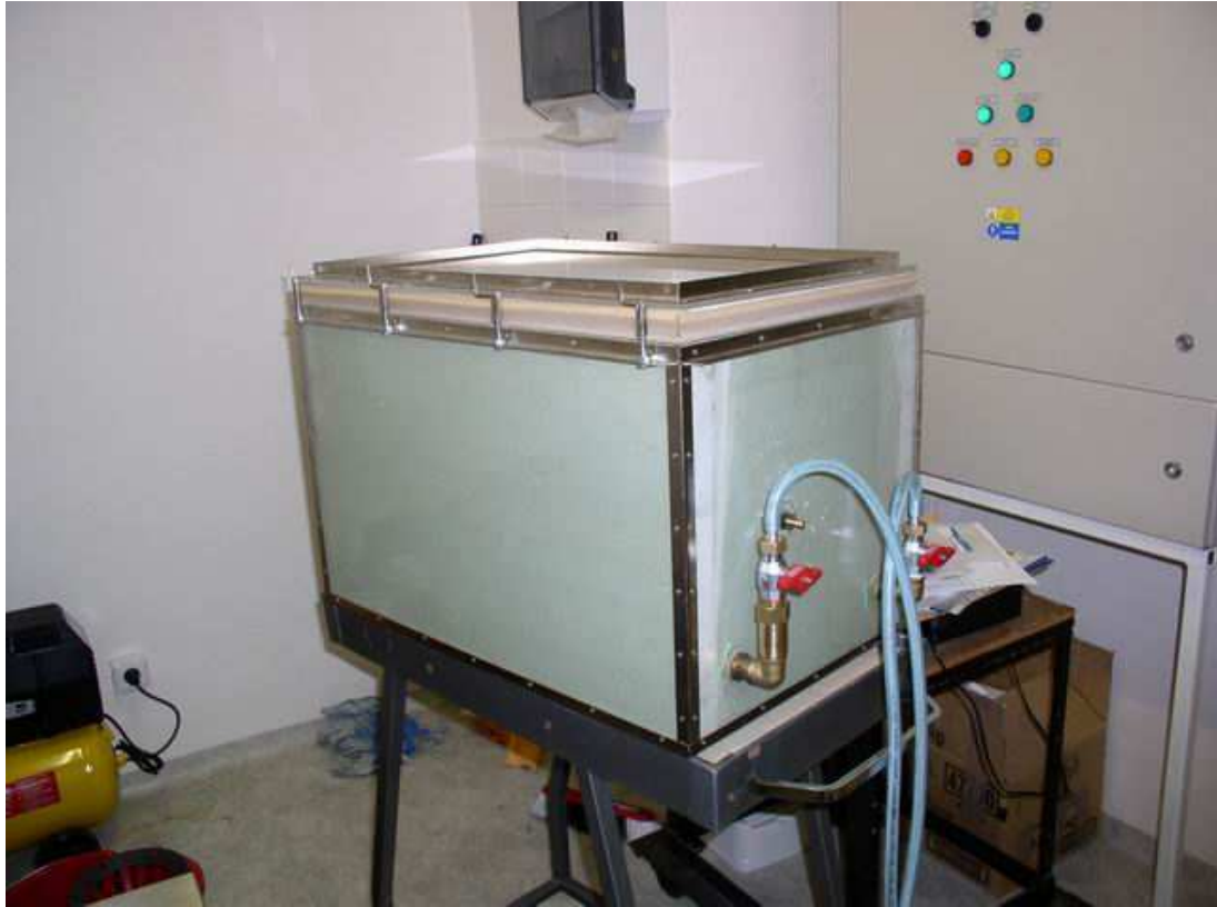
Figure 2a. Test box for six modules with cooling system, sensors and gas distribution
