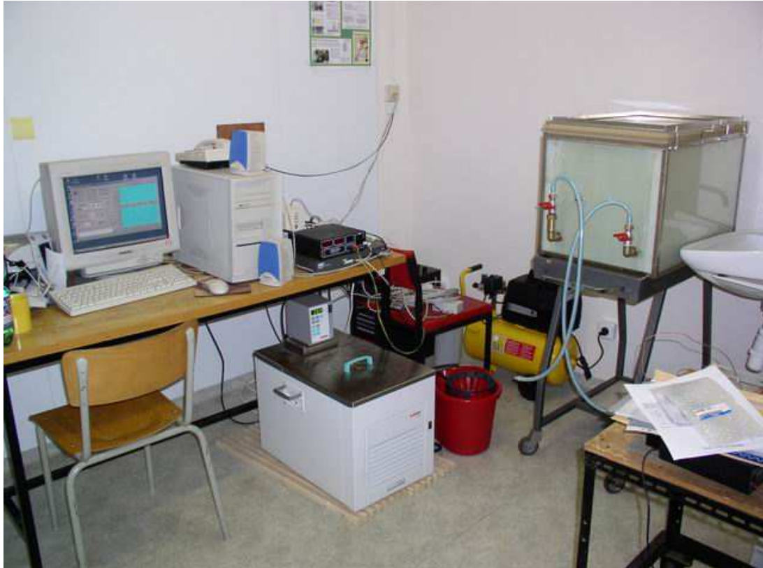
Figure 5. Charles University, Prague - grey room – general view to DCS control place with chiller “Julabo”, dry air source, sensors and test box for six modules
