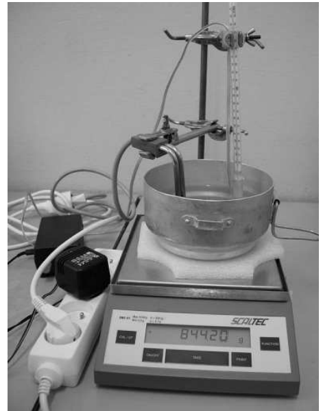
FIG. 6: The measurement of the evaporation speed: The immersion heater controlled by the simple switching circuit act as thermostat, the pot with water is regularly weighted.
