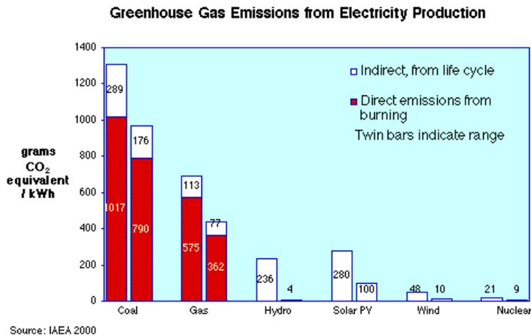
*Fig.2: Results of life-cycle analyses for CO<sub>2</sub> emission from electricity generation by various methods (Source: [5])*
